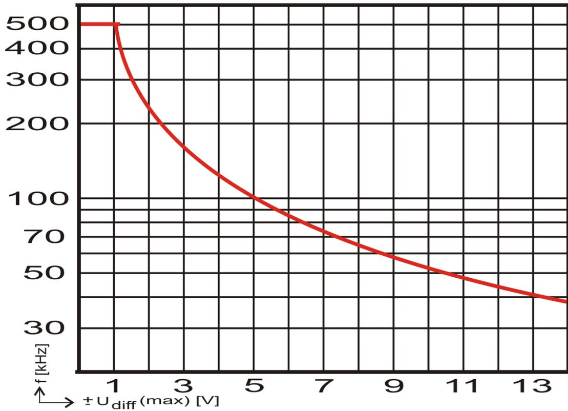
Fig. 4.1. – Differential input range
