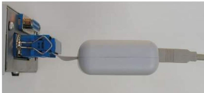
Fig. 1.2.5.1: How to connect the USB adapter
